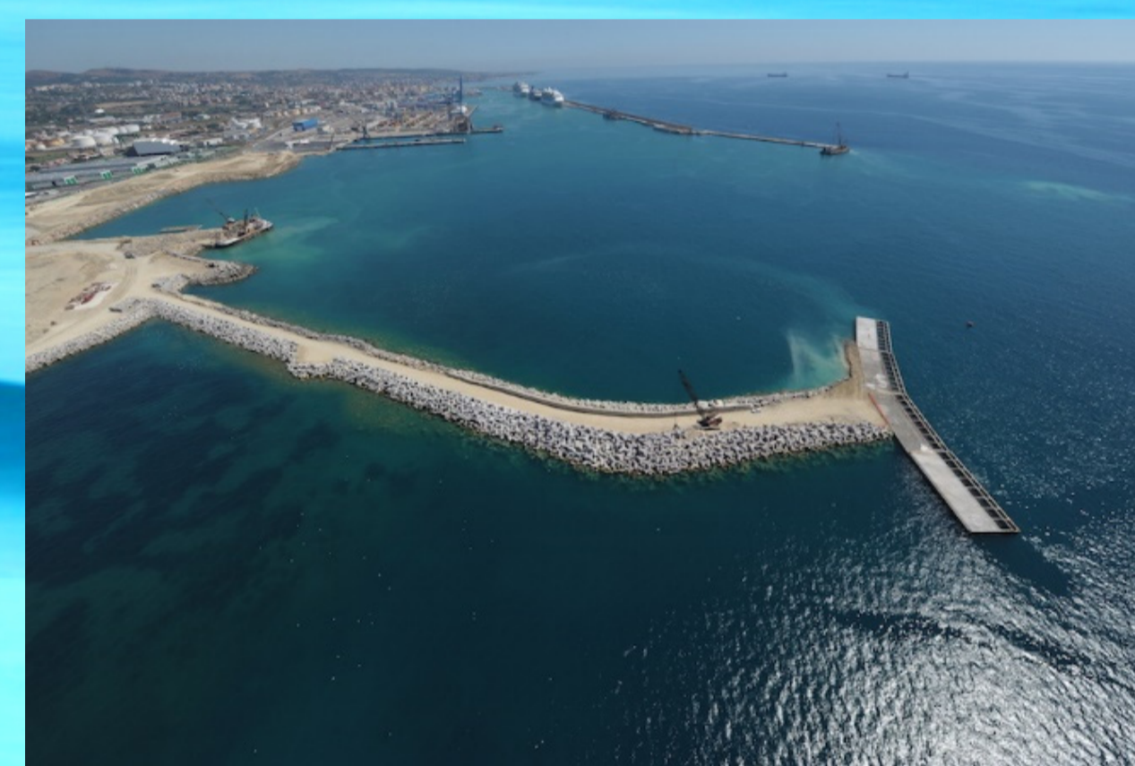
Figure 2. REWEC3 - Resonant Wave Energy Converter, commissioned in 2012 in Civitavecchia, Italy. Photo by www.Duomi.it.
